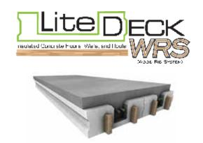
Mostly used in residential applications, the LiteDeck Wood Rib System is a carpenter friendly formwork for jobsite fabrication and concrete forming. Locally available lumber is used in the rib to support the weight of concrete. The wood rib can be removed after placement of concrete to be reused within the construction of the structure. Custom designs and pre-assembly are additional options.
