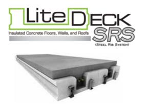
LiteDeck Steel Rib System is typically used to achieve large clearspans for floors, roofs, decks and tilt-up applications. This formwork is manufactured to job specific specs and is available in 40+ foot lengths. 18 gauge steel ribs offer tremendous fastening strength and are fire resistant. The steel rib can be cut out and removed after placement of concrete to be reused within the construction of the structure.
